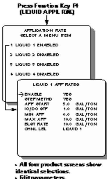
1. From the keyboard, press F4 to obtain the LIQUID APPLICATION RATES screen (See Figure 28).
