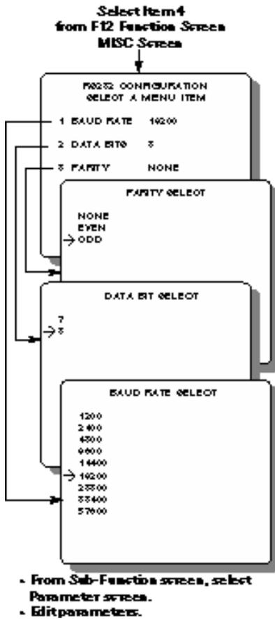
5. Select F12 to return to the MISC Menu and select SERIAL PORT CONFIGURATION using the 4 key. (See Figure 19).
