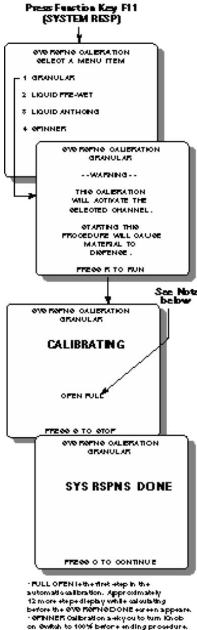
These constants adjust the response time of the Control Point™ system to the hydraulic and mechanical systems. This procedure determines the System Response (SYS RSPNS) and related constants (VALV BOOST, PWM OFFSET, PWM SAT, and AFILT) for each of the three control channels (granular, liquid, and spinner).
