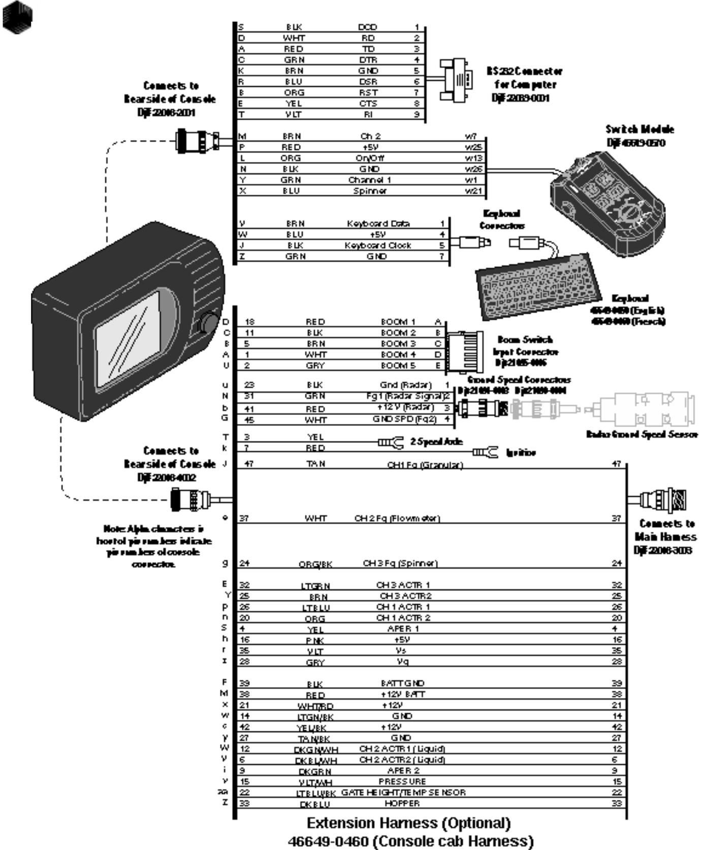
Figure 44. System Wiring Diagram, Console and Cab Harness
