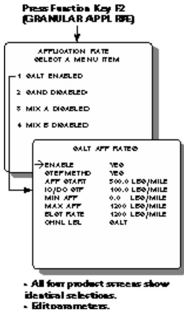
The APPLICATION RATE menu lists four granular materials. Each material screen contains a set of values for product application rate, APR steps, min/max limits, and blast rate. The pre-programmed values are usually the same for all granular materials but may be edited and modified as required.
