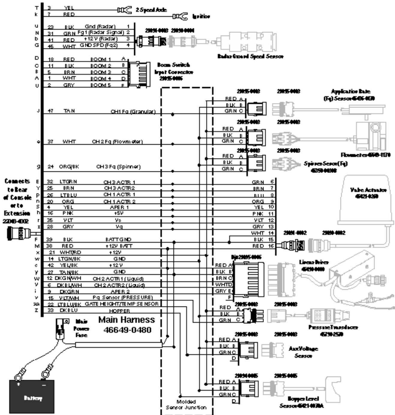
Figure 45. System Wiring Diagram, Truck Harness and Sensors
